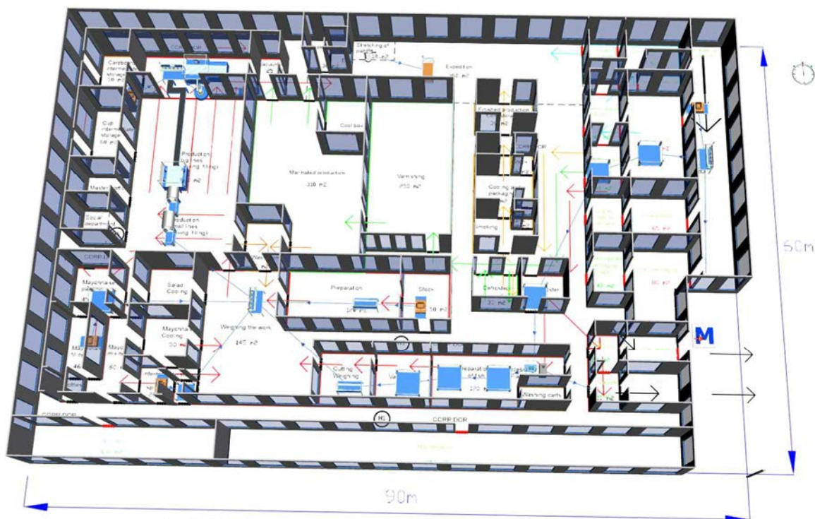
Figure 4 3D model of the production process of Treslovakian Cod
