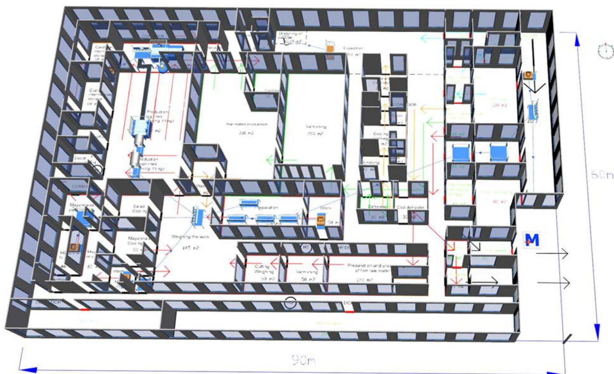
Figure 5 3D model of the Paris salad production process
