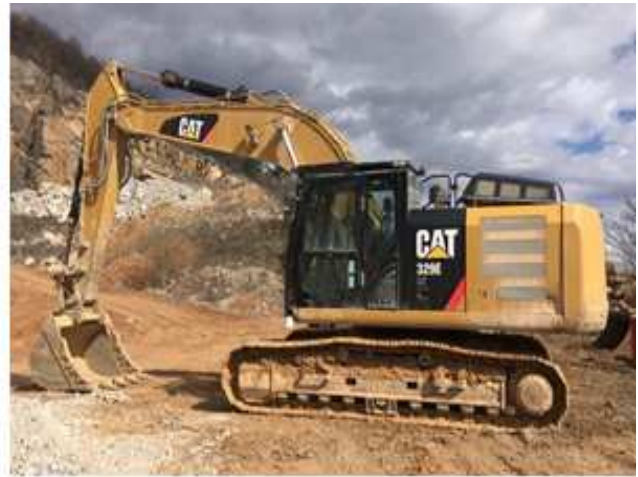
Tracked excavator CAT329F
