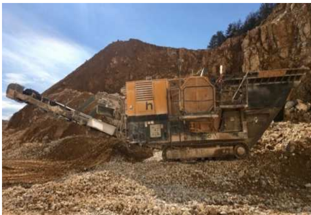
Crusher Hartl Powercrusher 12/65J
