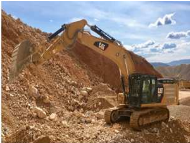
Tracked excavator CAT336F
