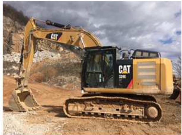
Tracked excavator CAT329F
