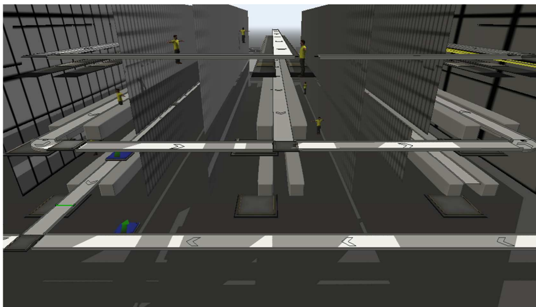
Figure 4 Flexsim representation of the multi-storey warehouse
