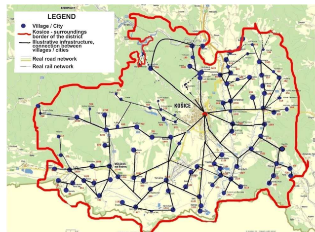
Figure 1 The structure of the road network in the Kosice – surroundings district
