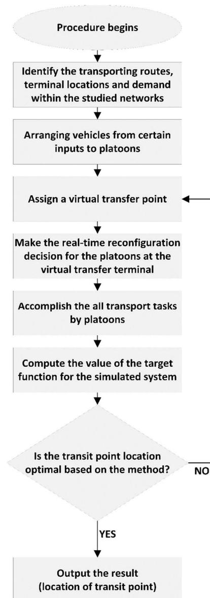
Figure 6 Virtual transfer point optimization in Physical Internet network
