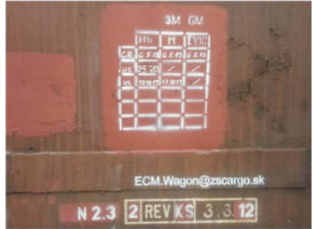
Figure 4 The current state of recording technical inspections
