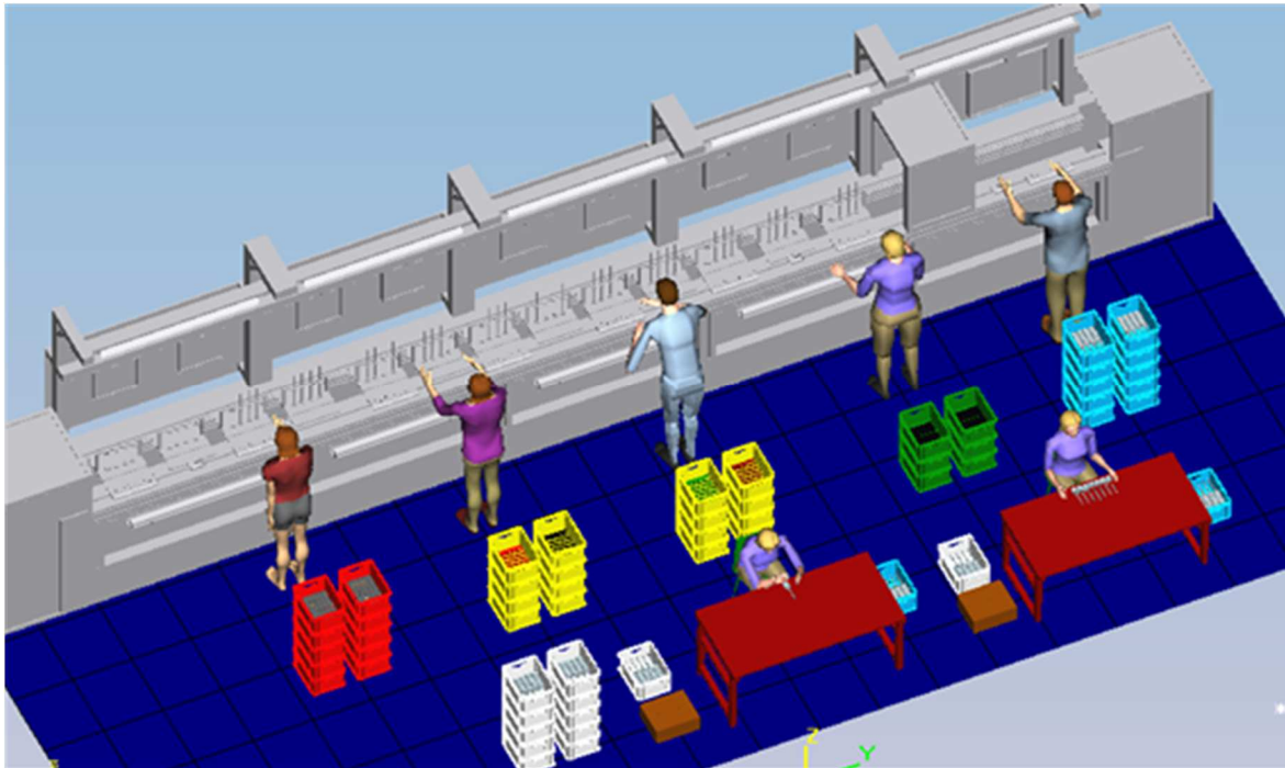
Figure 6 Proposal of production process layout with production line in Process Designer
