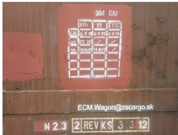
Figure 4 The current state of recording technical inspections
