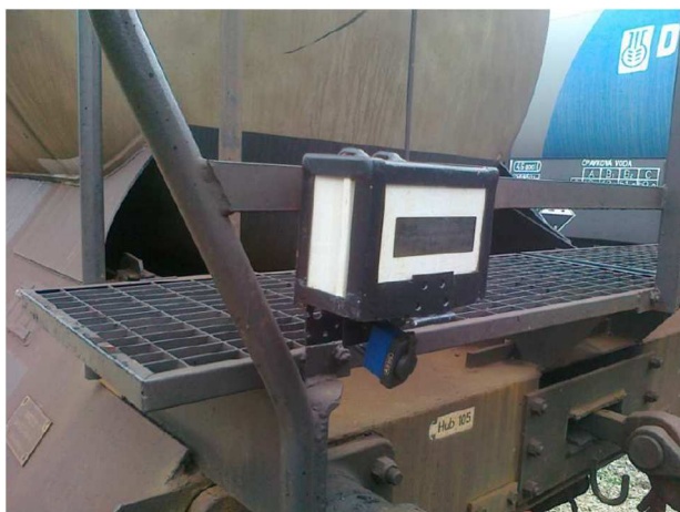
Figure 1 GPS tracker in box on a rail wagon
